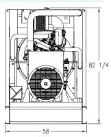
Drawing above for illustration purposes only, based on standard open power 480 volt generator. Lengths may vary with other voltages. Do not use for installation design.
